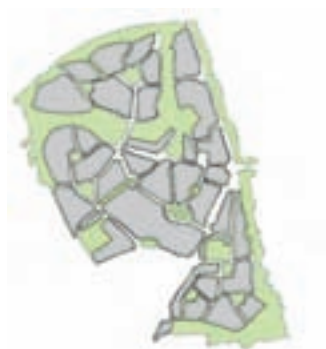
The proposed Ashton Green urban extension in Leicester comprises an irregular or deformed block structure
