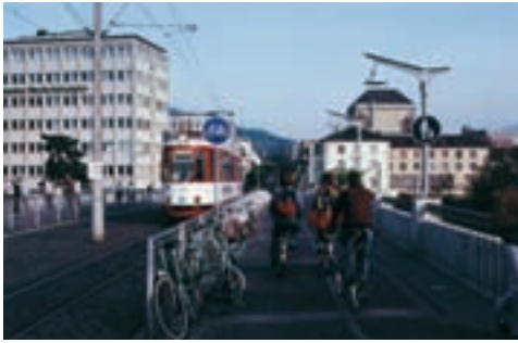
A bridge giving access to the town centre over the railway is for trams, cycles and pedestrians only. Freiburg, Germany.
