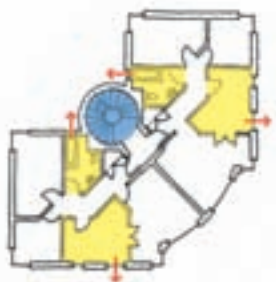
The rooms needing the most maintenance and refurbishment, bathrooms and kitchens, should be located to make change easier (proposed house type for Trowbridge Estate redevelopment, Hackney: PRP Architects)
